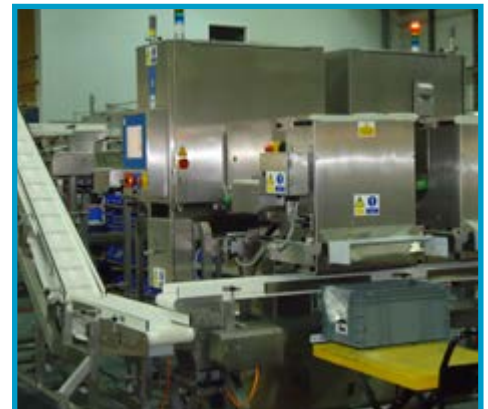
Dual X-ray system inspecting loose chicken fillets
