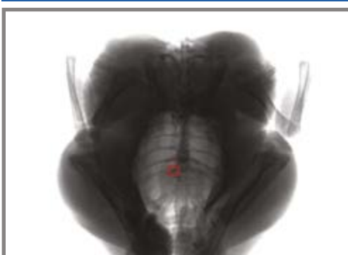
X-ray system finds stainless steel within whole chicken
