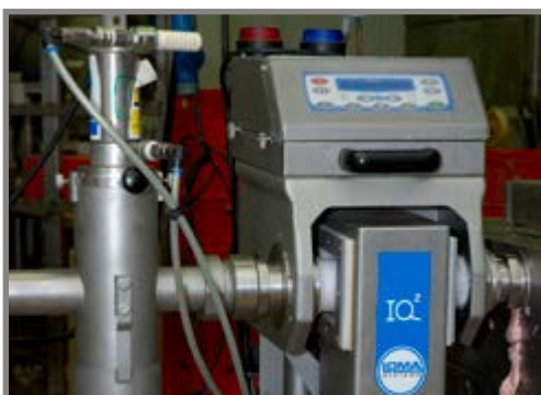
Pipeline system detecting metal in meat slurries prior to stuffing
