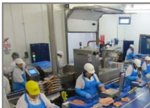
Combo system detecting and weighing processed poultry
