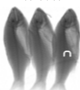
Staple identified in fish packed on foil board
