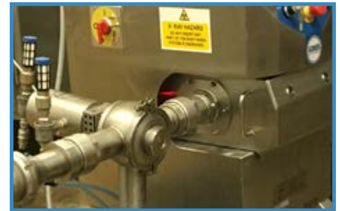
ARL Rotary reject valve used for inspecting whole muscle meat on the X5 Pipeline
