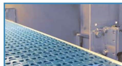
Reject Confirmation Sensor checks the pack enters the bin correctly
