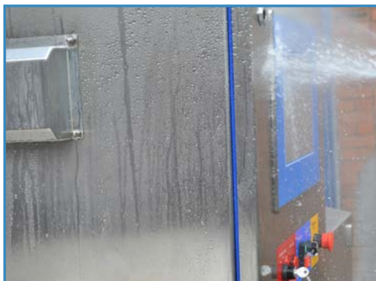
Low-pressure washdown of X-ray system
