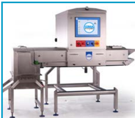
X5 Bulkflow scans fast-flowing loose product
