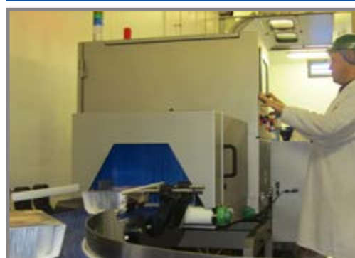
X-ray system inspects foil tray packed meat joints
