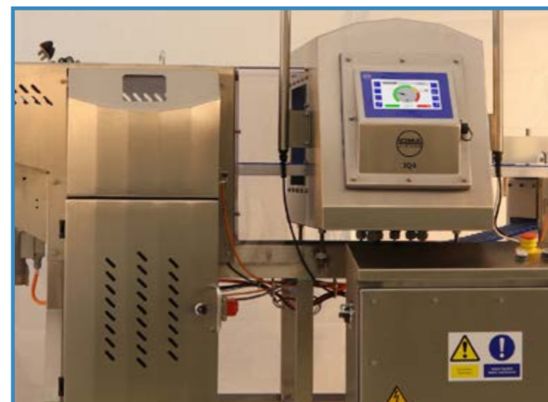
IP69K rated metal detector system for high pressure harsh washdown cleaning
