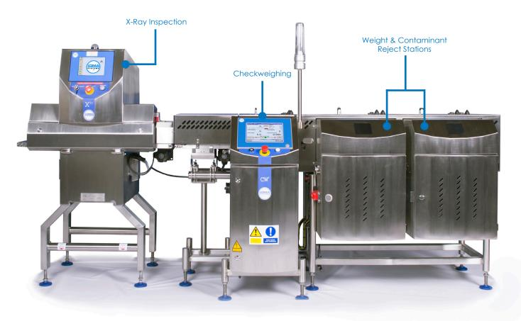
X5C Compact X-ray and CW3 Checkweigher Combination System
