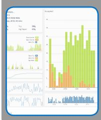
Developed in partnership with AutoCoding Systems, LOMA TRACS is a software application that provides centralised real-time data management capability. It requires a system to be connected via Ethernet to a central server and provides reporting of a range of current and historic batch information, including across multiple machines.
